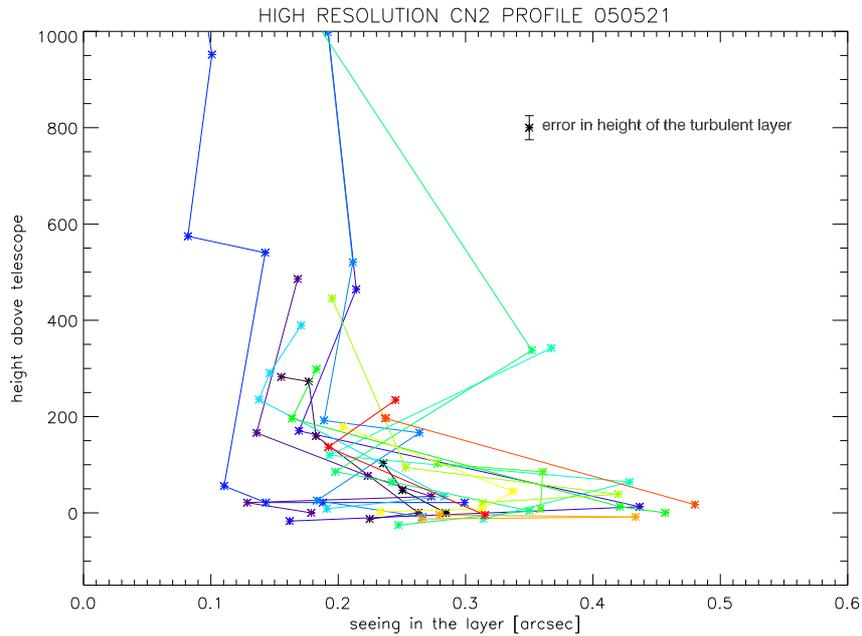
**Figure 5.** The seeing in the single layers as retrieved from the data of 21 May 2005. The vertical resolution is  $\approx 25\text{m}$  (as indicated by the error bar). A weak layer is located just above the VATT, and the two major layers are located at 50m (by far the strongest layer) and 350m above the ground. The colors corresponds to different cross-correlation images taken during this night.
