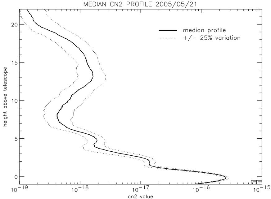
**Figure 1.** The median  $C_N^2$ -profile as measured with a Generalized SCIDAR in standard configuration for one night. The turbulence profile has a vertical resolution of around 1km, and no inner structure of e.g. the ground-layer peak can be seen.
