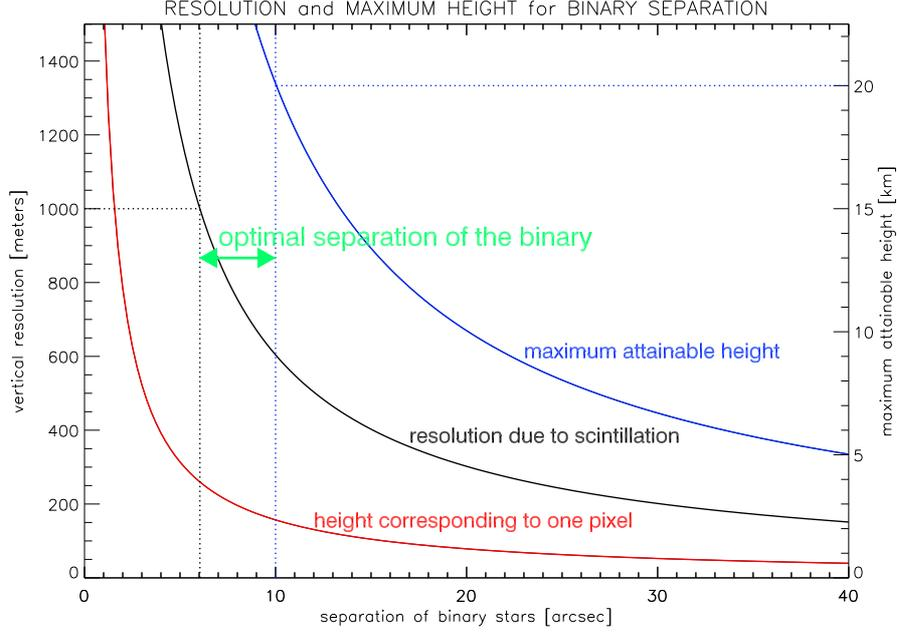
**Figure 2.** The achievable vertical resolution at the ground and the maximum attainable height above the conjugation plane of the detector versus the separation of the binary used for the SCIDAR observations. By choosing reasonable numbers for the desirable resolution at the ground and the maximum altitude, the range for the optimal separation of the binary for normal operation of the Generalized SCIDAR is for a telescope of 1.75m diameter between 6 and 10 arcsec.
