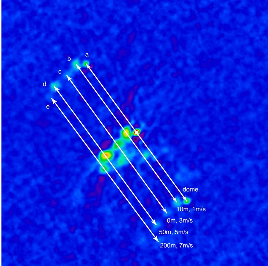
**Figure 3.** Sample cross-correlation image of  $\beta$  Cyg. For the detected triplets, the retrieved heights above the telescope and the wind speeds are indicated. The uncertainty in the height of the single layers is around 25 meters.
