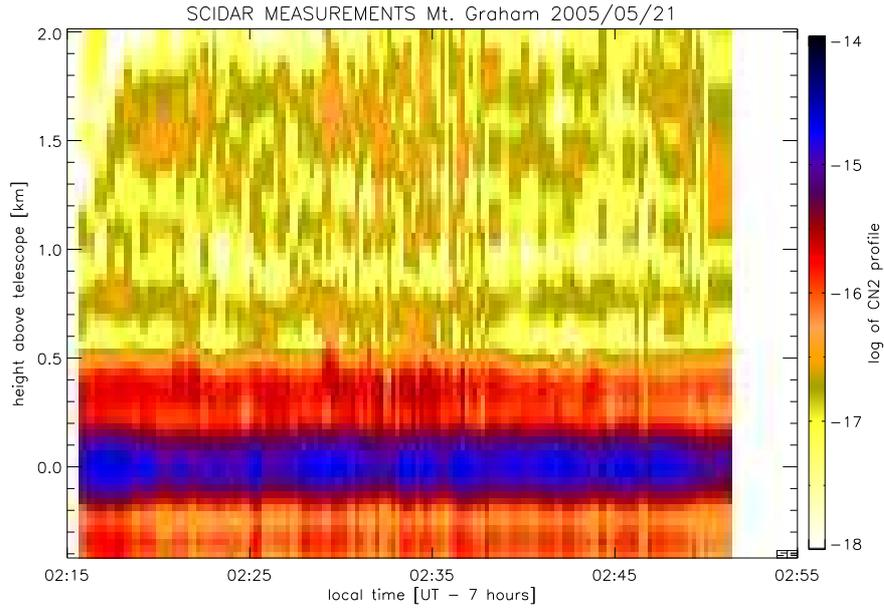
**Figure 4.** The temporal evolution of the  $C_{N,ac}^{2*}(h)$  profile as determined from the auto-correlation images when using a wide binary with a separation of  $35''$ . According to figure 2, the maximum attainable height above the telescope is limited to around 2 km, and the vertical resolution is around 200 meters (as can be seen in the thickness of ground-layer turbulence).
